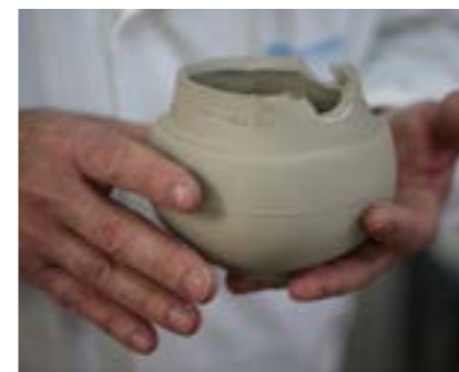
The hand casted bowl, still in soft clay, is born out of the mould.
