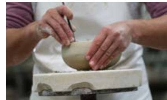
The leftover material is being removed, and the bowl must dry before firing in the kiln.
